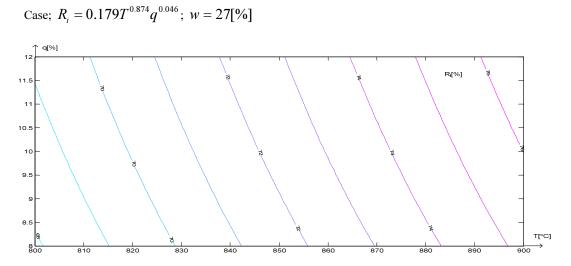
Figure 5: Percentage's Dependency of Pre-Reduction Degree (Ri) from Temperatures and Ancillary Material for Humidity Level 27%
