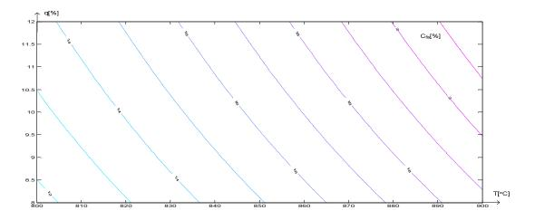
Figure 4: Percentage's Dependency of Pre-Reduction Degree (Ri) from Temperatures and Ancillary Material for Humidity Level 22%
