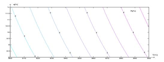
Figure 3: Percentage's Dependency of Pre-Reduction Degree (Ri) from Temperatures and Ancillary Material for Humidity Level 22%
