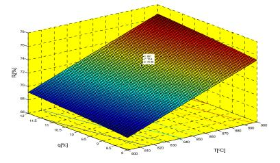
Figure 1: Regression Surface for Dependence of Pre-Reduction Degree of Nickel Ores from Temperature and the Amount of Ancillary Material (Kosovo Lignite and the Stone Coal Indonesia)
