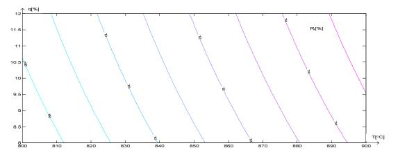
Figure 7: Percentage's Dependency of Pre-Reduction Degree (Ri) from Temperatures and Ancillary Material for Humidity Level 32%
