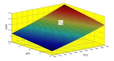
Figure 2: Regression Surface for Dependence of C<sub>fix</sub> from the Amount of Ancillary Material and Temperature
